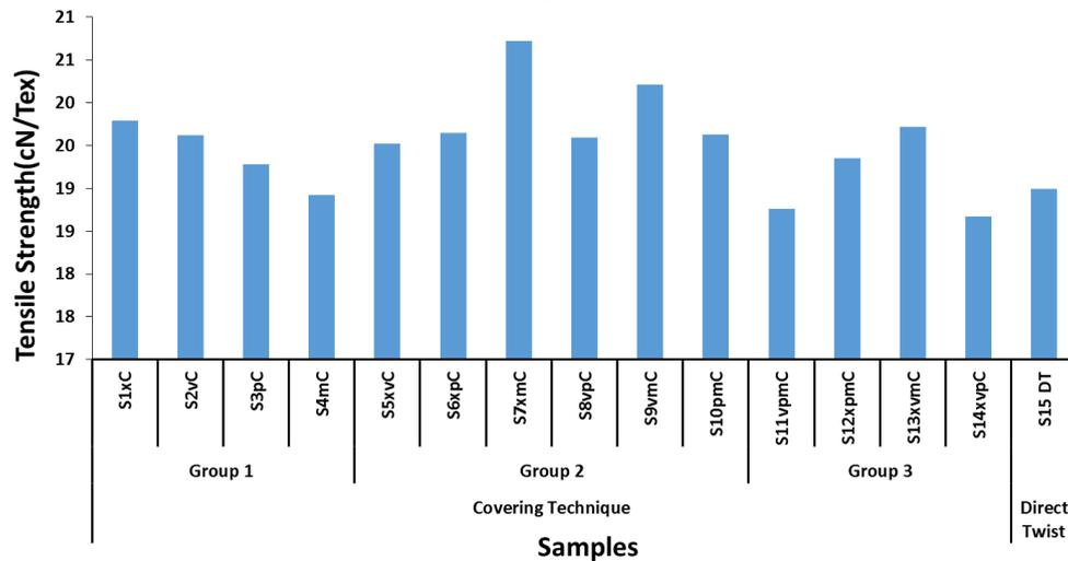
Figure (1) Results of yarn Tensile Strength (cN/Tex)
