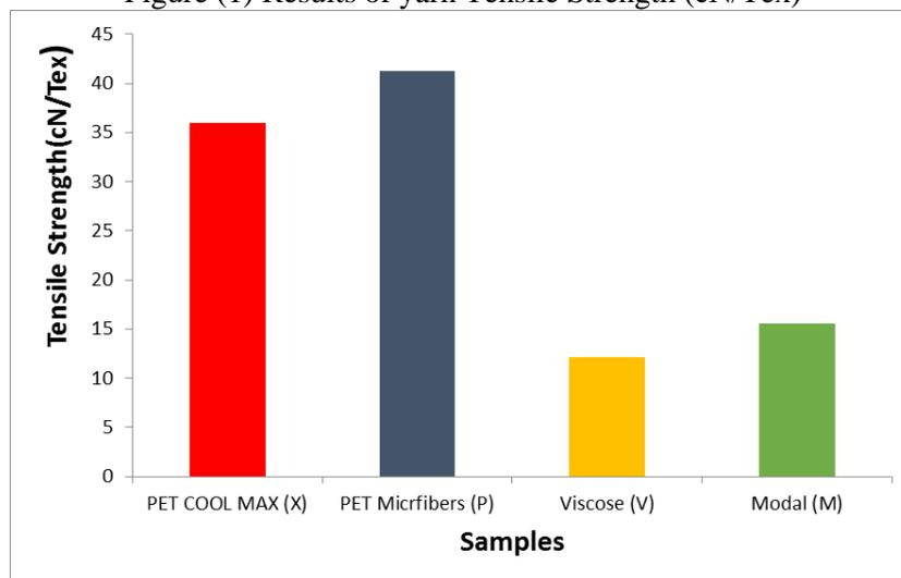
Figure (2) Results of yarn Tensile Strength (cN/Tex) to original samples
