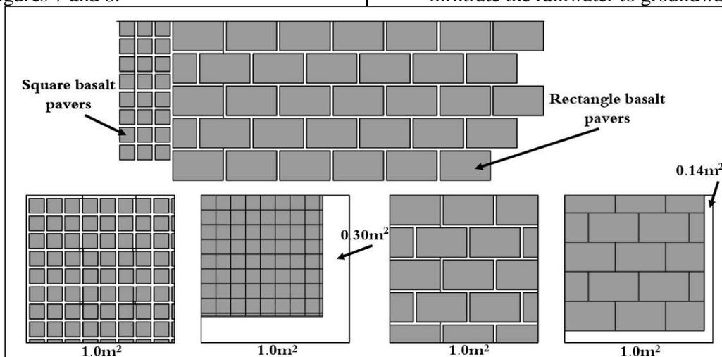
Figure 6. the porosity of two types of basalt pavers of El-Moez street, source: the researchers.
