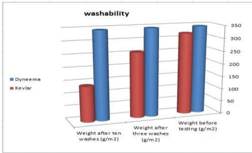
**Figure 8. Weight before and after washability Test**
