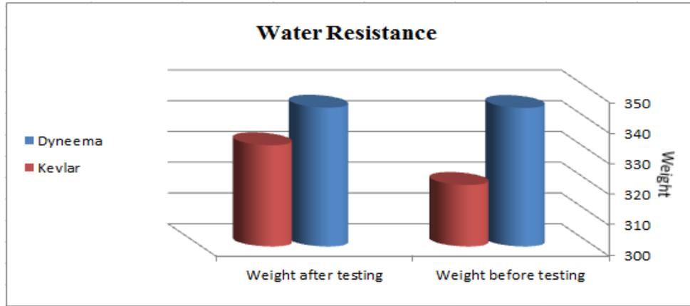
Figure 6. Weight before and after Water Resistance Test
