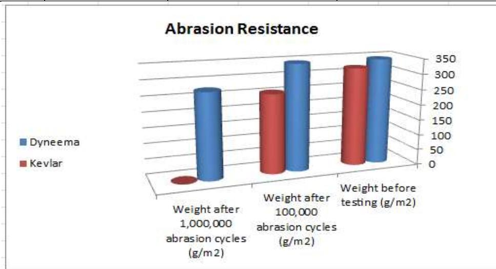
Figure 7. Weight before and after Abrasion Resistance Test
