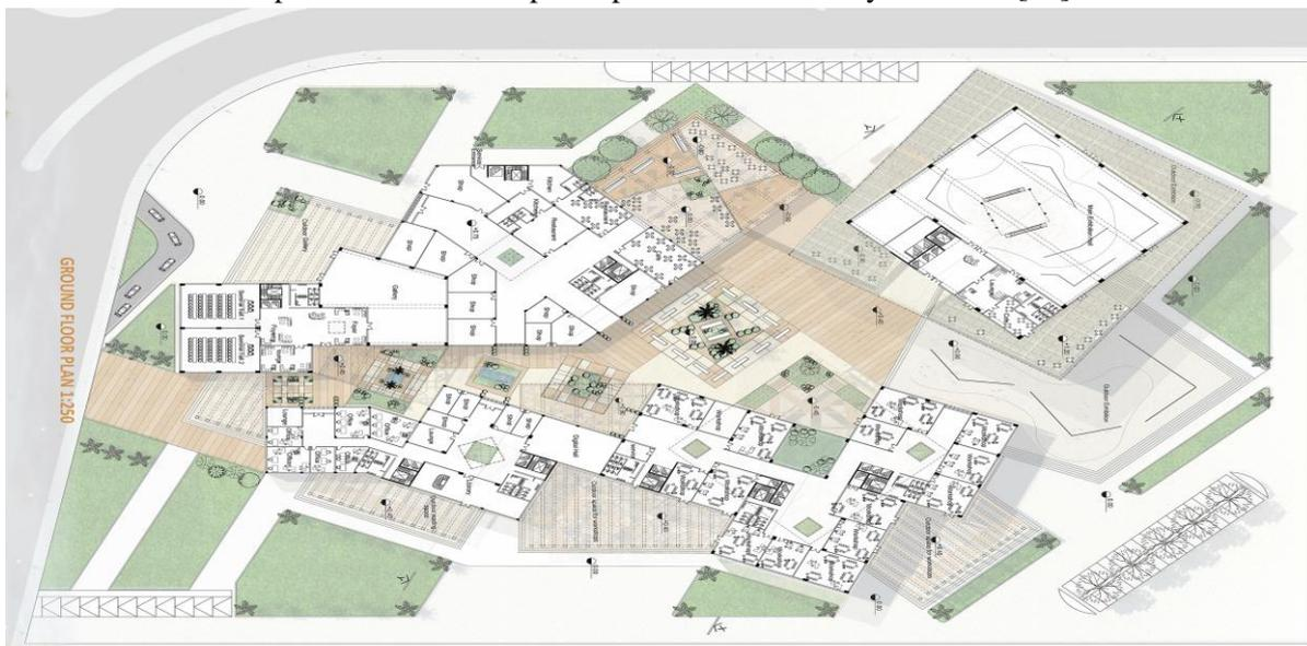
Fig. (54) The floor plan of the vocational training center which consists of the entrances, the commercial area, the main courtyard of the project, workshops and the main hall.
