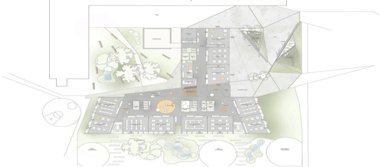
**Fig. (39)** the vocational training center floor plan which shows the interior spaces, corridors and services.
