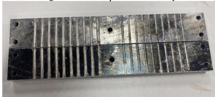
**Figure 2 Aluminum Mold**
