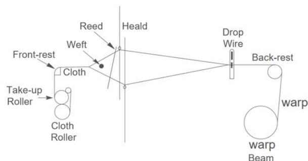
Fig.2 Passage of warp yarns through the loom
