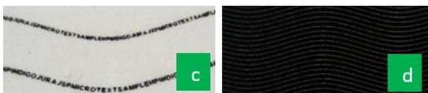
**Figure (3):** a) Linework, b) Microtext at 0.8 pt, c) wave-text at 1.0 and 0.8pt, d) knockouts elements (HP 6K guide)
