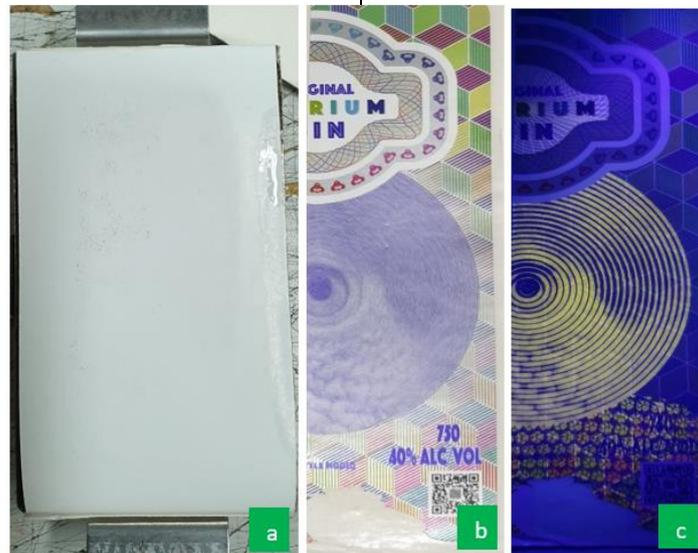
**Figure (14):** a) Design 2 Group A wetted test result (blank paper) after 25 stroke sequence, b) design 2 Group A sample visible ink after wetted rub test, c) design 2 Group A sample invisible ink after wetted rub test
