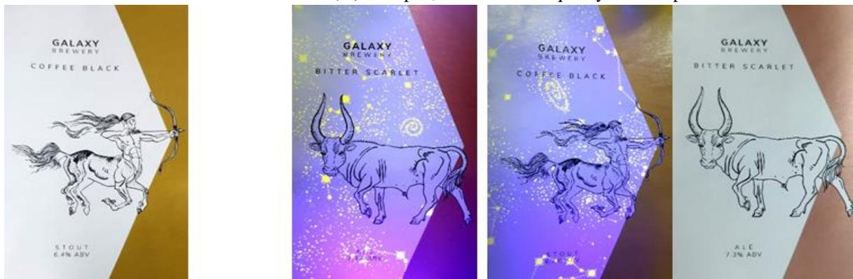
Group B, The Printed Design Label 2 before UV exposure Group B within UV exposure Figure (6): the printed design 2 experiments Group B / security covert invisible design analysis by UV lamp source
