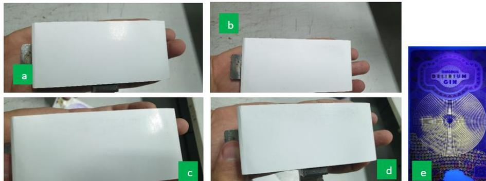
Figure (9): a) Design 2 Group A test result after 25 stroke sequence, b) Design 2 Group A test result after 75 stroke sequence, c) Design 2 Group A test result after 100 stroke sequence, d) Design 2 Group A test result after 150 stroke sequence, e) Design 2 Group A under UV light source after end of dry ink rub test
