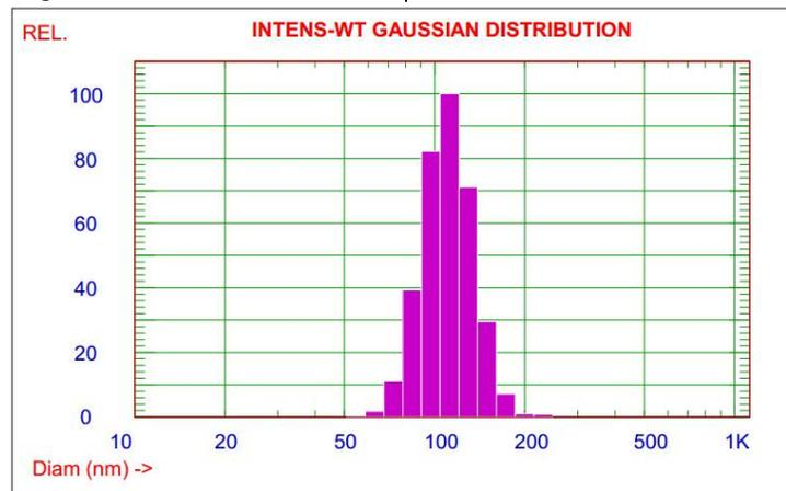
Figure (2). illustrated the particle size distribution of polystyrene/hydroxy methacrylate copolymer/SiO<sub>2</sub> nano Coating
