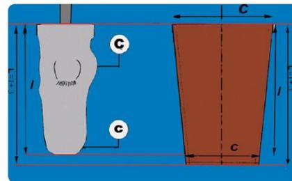
**Figure (6) Soft Liner Manufacturing**
