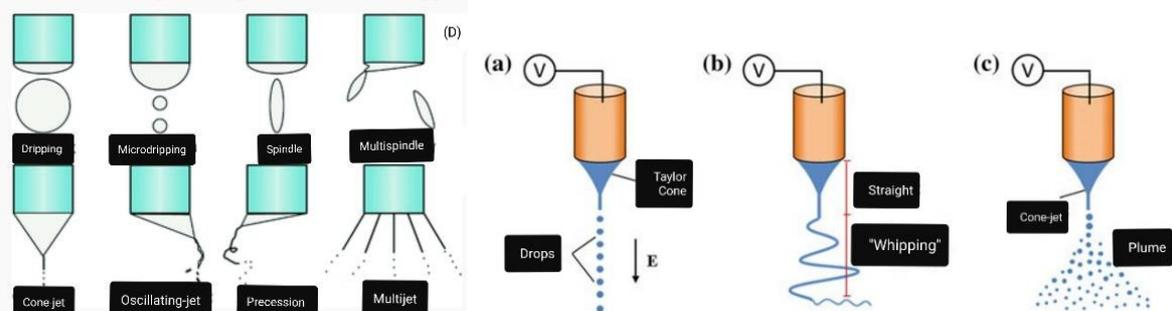
**Figure (6):** a) Schematic illustration of the E-jet printing, b) electrospinning, c) electrospaying, D) various modes of EHD writing.
