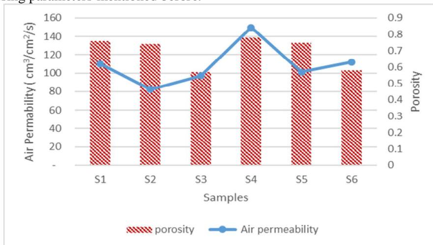
**Fig. (7) Relationship between air permeability & porosity**
