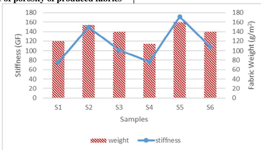
Fig. (9) Relationship between stiffness & fabric weight
