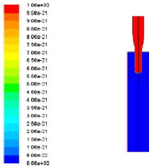
Fig. (16) Contours of water-liquid Volume Fraction After 6  $\mu$ s
