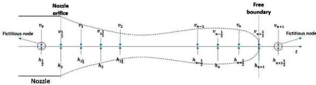
Fig. (1) uniform mesh of droplet formation (droplet connecting to nozzle )
