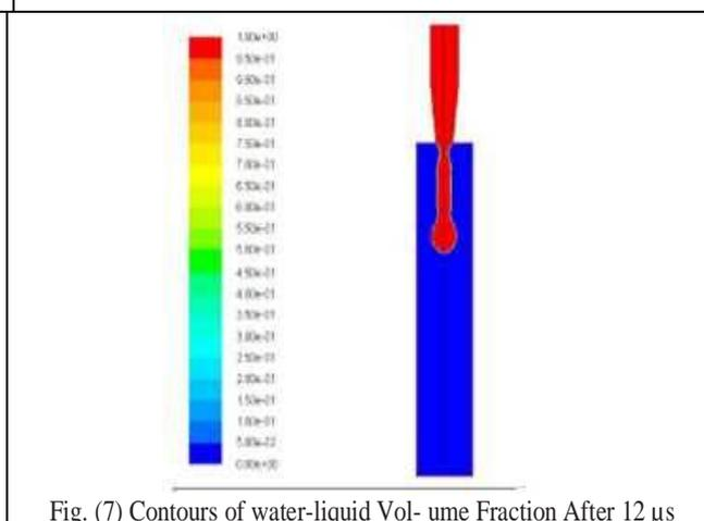
Fig. (7) Contours of water-liquid Volume Fraction After 12 μs
