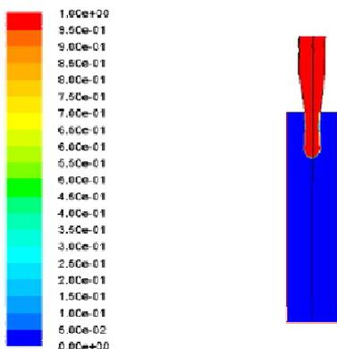
Fig. (21) Contours of water-liquid Volume Fraction After 6  $\mu$ s
