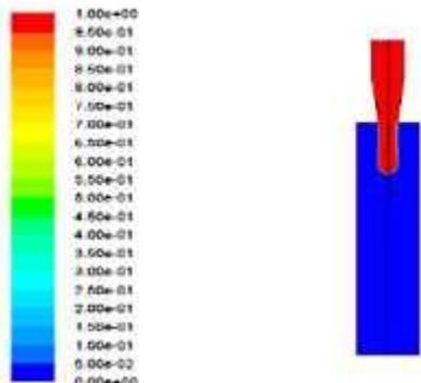
Fig.(10)Contours of water-liquid Volume Fraction After 30 $\mu$ s
