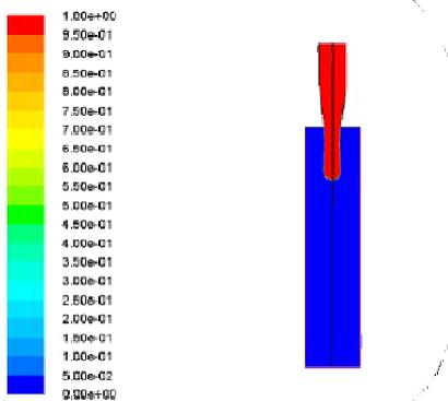
Fig. (26) Contours of water-liquid Volume Fraction After 6  $\mu$ s
