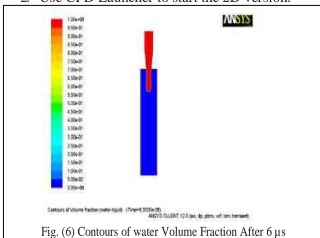
Fig. (6) Contours of water Volume Fraction After 6 μs
