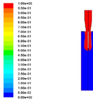
Fig. (27) Contours of water-liquid Volume Fraction After 12  $\mu$ s
