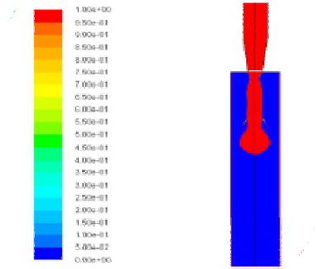
Fig. (23) Contours of water-liquid Volume Fraction After 18  $\mu$ s
