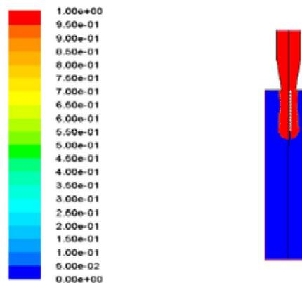
Fig. (22) Contours of water-liquid Volume Fraction After 12  $\mu$ s
