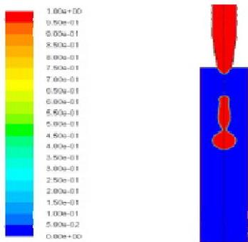
Fig. (18) Contours of water-liquid Volume Fraction After 18  $\mu$ s
