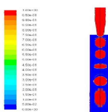
Fig. (29) Contours of water-liquid Volume Fraction After 24  $\mu$ s
