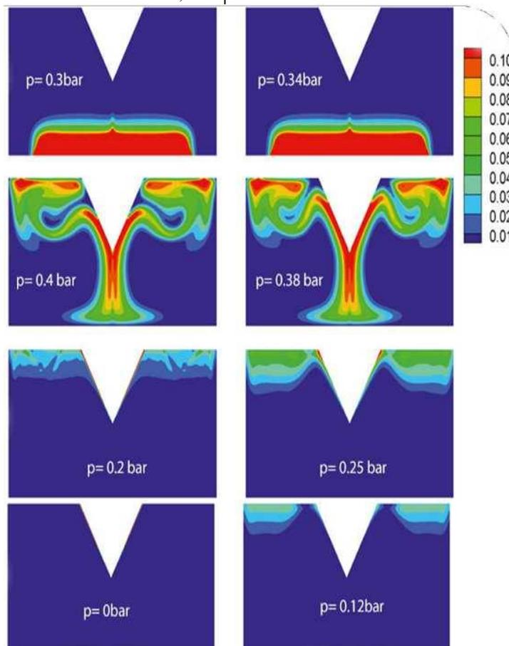
Fig. (5) Point shape during formation with different pressure
