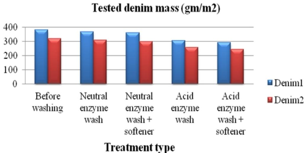
Fig.4: Tested denim mass before washing, after washing and after softening
