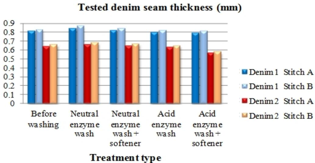
Fig.8: Tested denim seam thickness before washing, after washing and after softening
