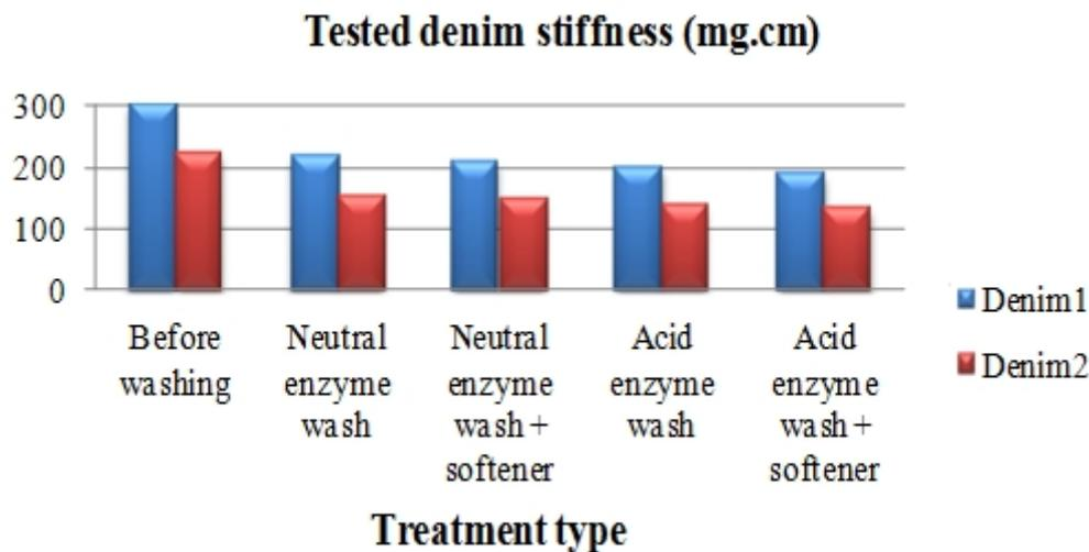
Fig.7: Tested denim stiffness before washing, after washing and after softening
