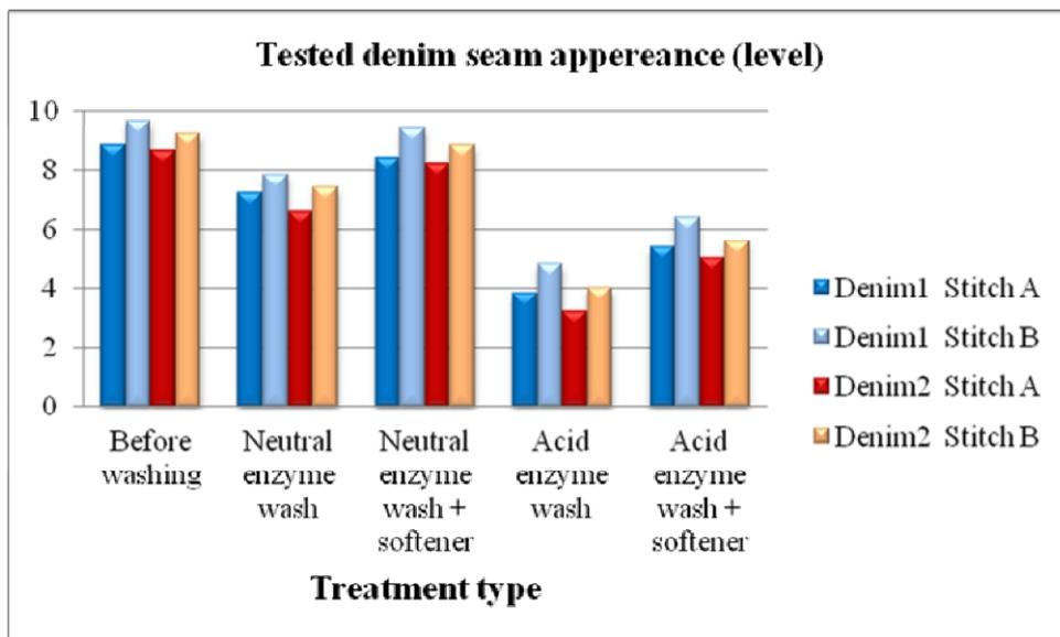
Fig.11: Tested denim seam appearance before washing, after washing and after softening
