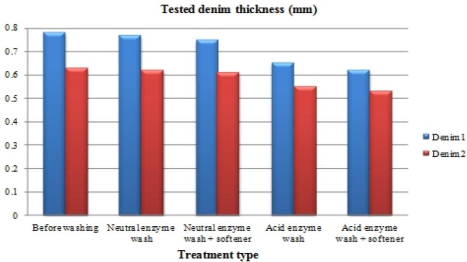
Fig.5: Tested denim thickness before washing, after washing and after softening
