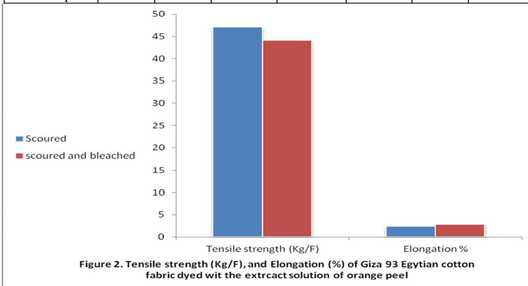
Figure 2. Tensile strength (Kg/F), and Elongation (%) of Giza 93 Egyptian cotton fabric dyed with the extract solution of orange peel
