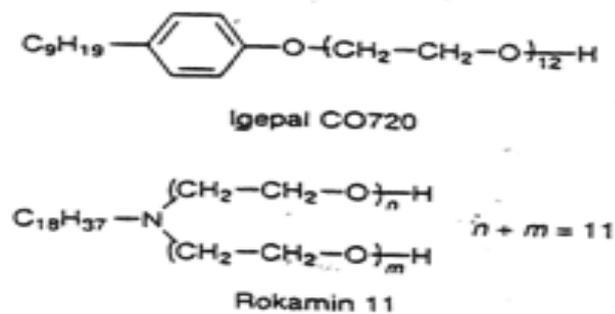
Figure 2. Chemical formula of nonionic surfactants Igepal CO720 and Rokamin 11
