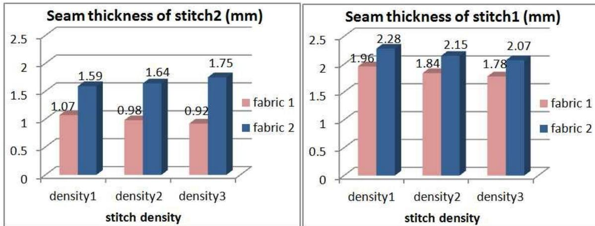
Fig(5) Seam thickness of tested fabrics
