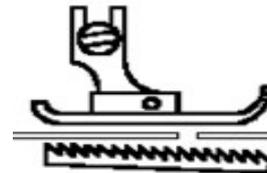
(c) Position of the feed dog with its side opposite the operator in a raised position.
