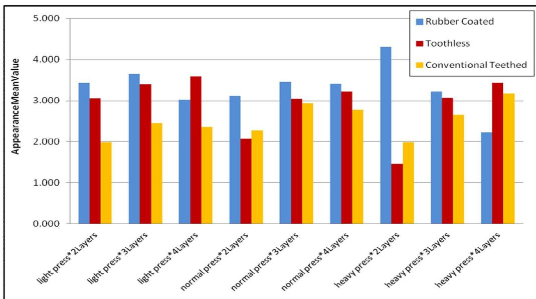
Figure (12): Effect of using modified feed-dogs on mean values of appearance test
