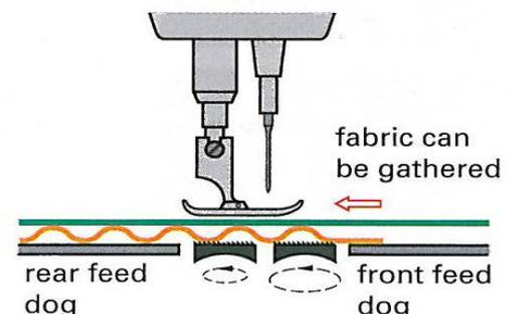
Figure (2): Differential feed mechanism
