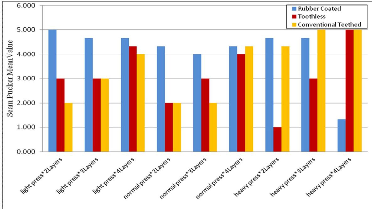
Figure (13): Effect of using modified feed-dogs on mean values of seam pucker test
