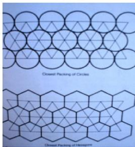
Fig 10: Triangulation of two-dimensional closest packed arrays.
