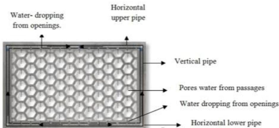
(Fig 29) In summer; a frontal sector to show how the water drops directed from the hexagonal horizontal passages to horizontal lower pipe, to vertical pipes then dropping once again from the horizontal upper pipe
